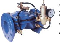
RAF valves made of only three parts, each one made of durable materials. The inner flow passages are streamlined and coated with low-friction materials. This provide quiet flow in both directions, flow head loss and minimal wear. RAF valves operate with a patented reinforced diaphragm, which eliminate the need for a retaining metal spring.
