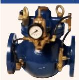
The valve automatically reduces a greater upstream pressure to a steady lower downstream pressure. The downstream pressure is governed by a pilot and can be adjusted. Downstream pressure is maintained at a steady set pressure regardless of changes in inlet pressure or flow rate. Minor changes in downstream pressure will immediately cause the valve to open or close accordingly, returning the system to a preset.
