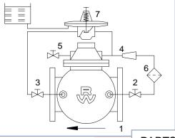
The altitude control valve automatically maintains liquid level in water tanks, reservoirs and storages at its maximum preset point. The valve is pilot controlled, and operates by comparing the water column pressure to the spring adjustment. The valve will be fully closed when the water reaches its preset level. The opening level is determined by the spring selection and varies from 30 to 100 cm.
