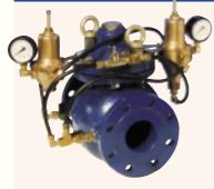
The valve performs both pressure reducing and pressure sustaining features. It maintains a constant upstream pressure to an adjusted value as a pressure sustaining valve, and reduces greater upstream pressure to a steady lower downstream pressure as a pressure reducing valve. Both functions occur independently, and the valve constantly modulates accordingly.
