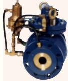
The purpose of the anti burst valve is to prevent water flow in pipes and systems that have been physically damaged from any reason. A high sensitivity flow pilot and an orifice plate, that indicates the current flow in the pipeline, control the valve. When a preset flow ("Burst" condition) is reached the valve will tight close. The valve can only be re-opened manually
