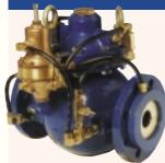
The valve maintains a steady flow rate at any working conditions. Regardless of pressure changes or demand, the valve will keep flow constant. The flow is controlled by a pilot and a calibrated orifice plate, and can be adjusted within a range of 20%. The orifice plate size is determined by the required flow range and is specific for each project.
