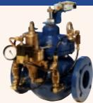
The pump control valve is made to protect pumps from possible damages caused by powerful start-ups and shutdowns of centrifugal pumps. The valve's purpose, is primarily minimizing the formation of surges during on/off operation of the pump, and protect pump from backflow. The valve is electrically interlocked with pump's control panel. Opening and closing speed can be adjusted, offering a smooth startup and shut-downs. By the action of a pilot The Pump
